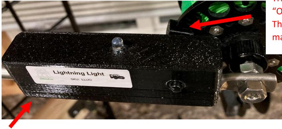
Trigger snaps into any "O" on the rattle reel. The side with the magnets faces the sensor.
