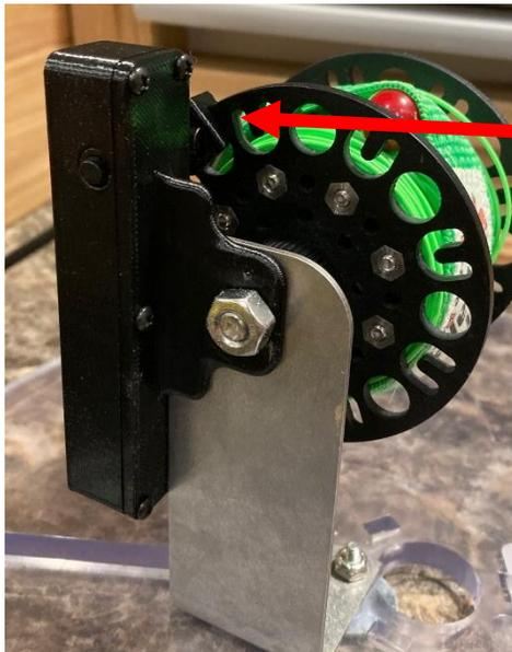
Trigger snaps into any "O" on the rattle reel. The side with the magnets faces the sensor.
