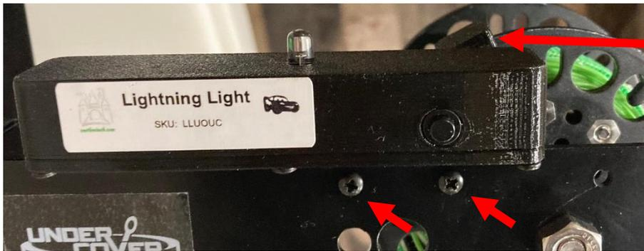
Trigger snaps into any "O" on the rattle reel. The side with the magnets faces the sensor.
